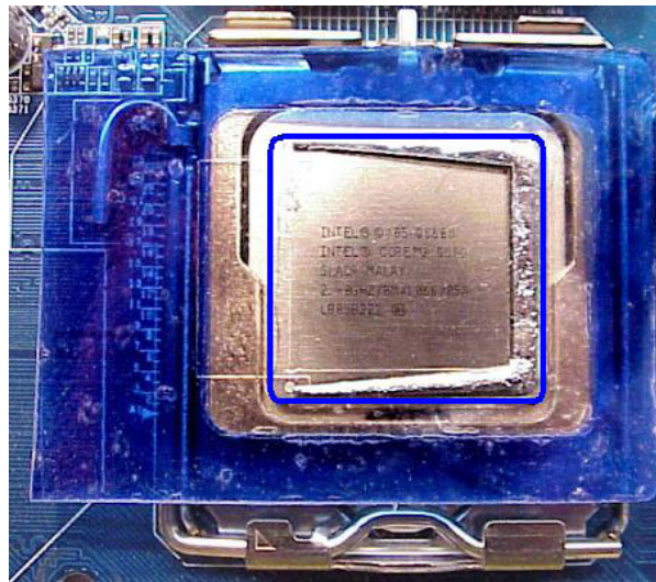
ETI on CPU lid with correct alignment and placement
